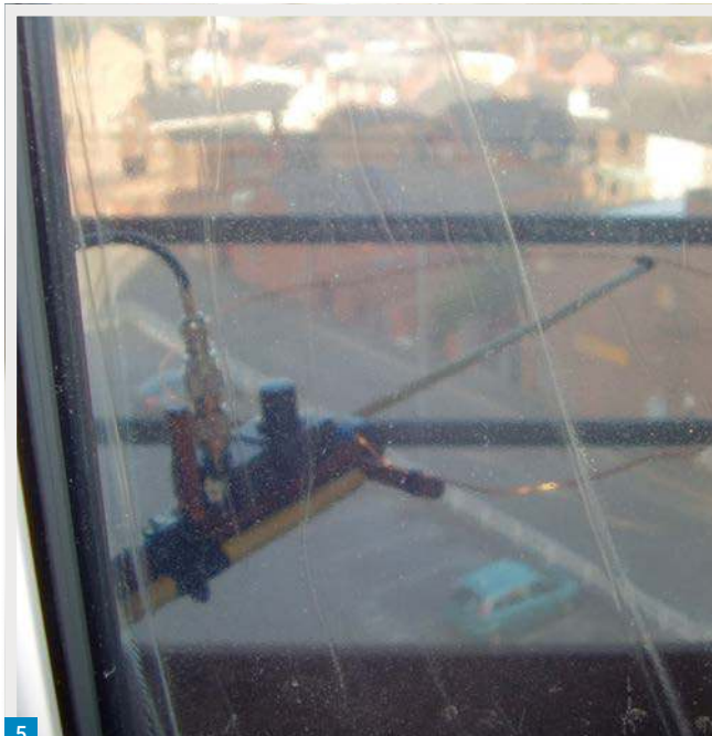
Fig. 3: The loop mounted on bamboo cane.
