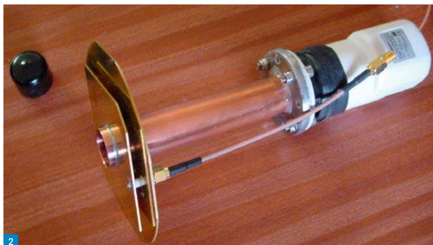
Photo 2: G3VKV's new dual-band feed for his QO-100 satellite station. Photo 3: G8BCG's QSO with Nauru on 2m EME.
