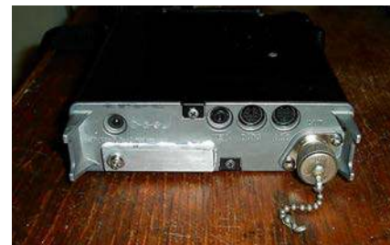
The additional heatsink in position.
